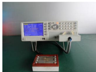
LCR DIGITAL ELECTRIC BRIDGE used for testing double common mode inductance and deviation
