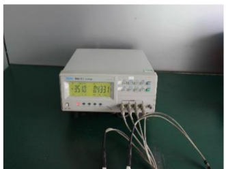
LCR DIGITAL ELECTRIC BRIDGE used for testing inductance
