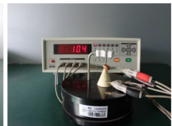
TOROIDE WINDING TURNS TESTER used for testing winding turns of toroide
